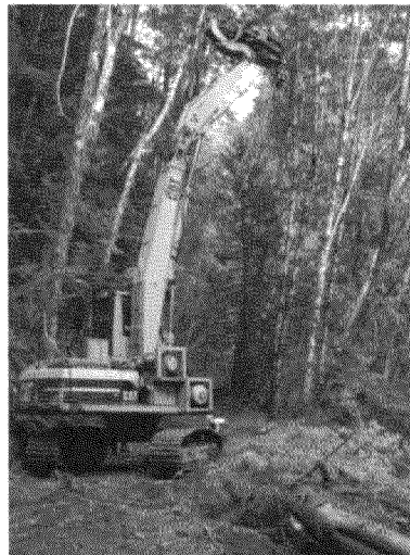
A yoader (combination log yarder/loader) selects logs to place in Lost Creek to improve fish habitat.
