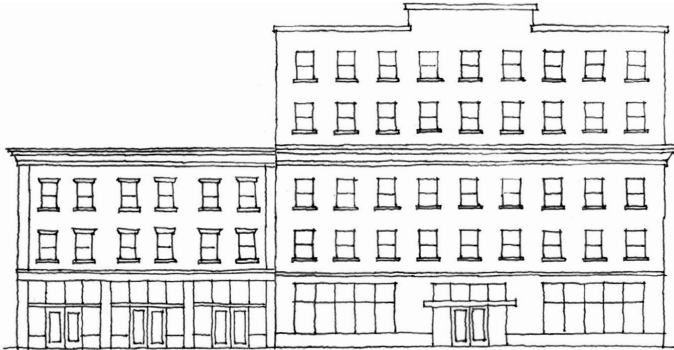
In this drawing of new construction (on right) next to a contributing building, the cornice line of the older building is reinterpreted into the façade of the new building.
