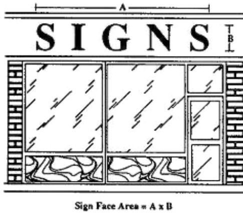
36.7505 Figure 4 – Sign Face Measurements
