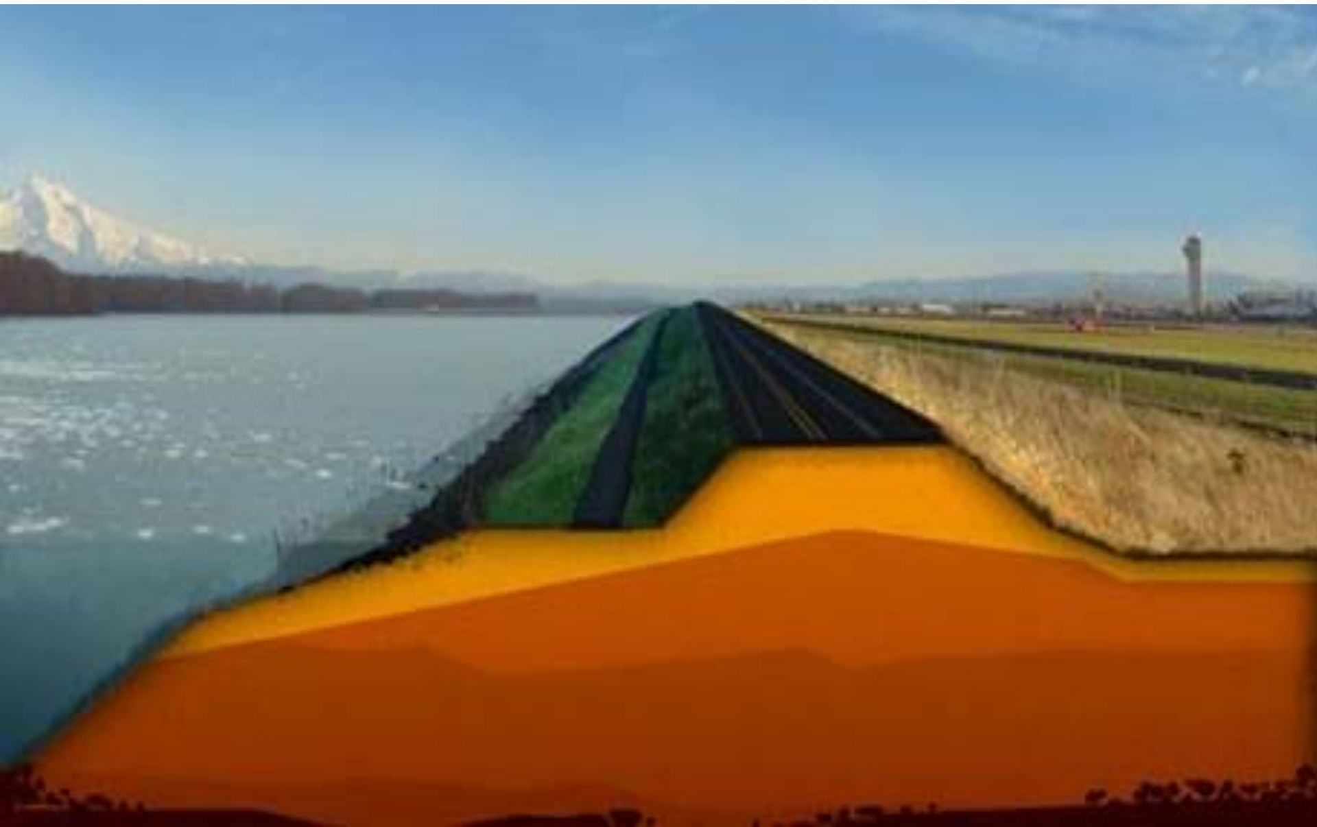
Levee Cross-Section along Marine Drive
