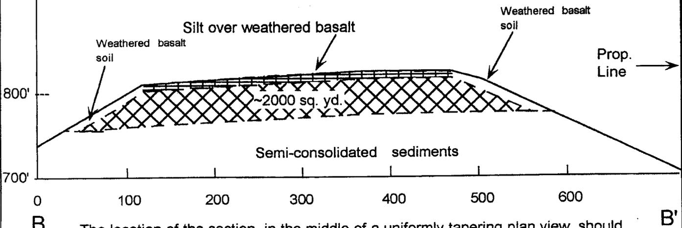
The location of the section, in the middle of a uniformly tapering plan view, should represent an average width.
