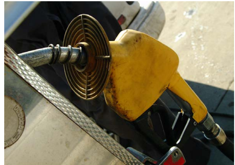
Odometer and other vehicle data uploaded when fuel nozzle inserted into tank
